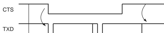
Figure 36-28. Transmitter Behavior when Operating with Hardware Handshaking
