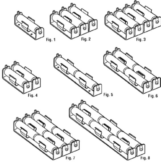
Holders: Available with solder lugs, PC lugs or series connections.
