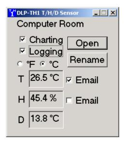
Since multiple DLP-TH1 units can be connected to the PC at the same time, when the program is run, the first required step is to select the sensor that is to be monitored. When the Open button is clicked, a selection window will appear that presents a list of all sensors connected to the PC. To select a specific sensor, simply click on the description string for the desired sensor and then click on OK.
