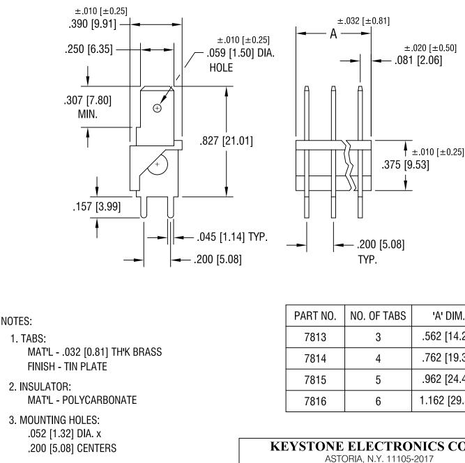
**KEYSTONE ELECTRONICS CORP.** ASTORIA, N.Y. 11105-2017 PART NAME .250 [6.35] PC QUICK-FIT HEADER MATERIAL AS NOTED DRN BY FINISH DATE BOONE 7 25 95 **TIN PLATE** APP'D SCALE LN 2X CHANGE AS PER ECN 05-006 D 2.1.05 DWG NO. TOLERANCES INCH [MM] CODE DECIMAL  $\pm .005 [\pm 0.15]$ 7813-7816 C/M ANGULAR  $\pm 1^{\circ}$ DATE DESCRIPTION REV. UNLESS OTHERWISE SPECIFIED
