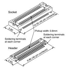
2. Strong resistance to adverse environments! Utilizes "**TDUGH CONTRET**" construction for high contact reliability. 3. Simple lock structure provides tactile feedback to ensure excellent mating/unmating operation feel.
