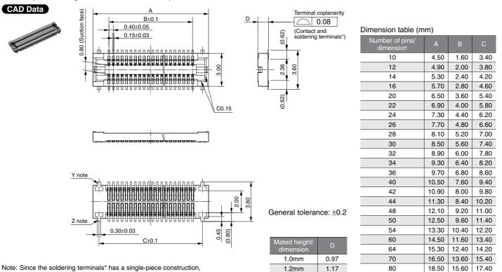
sections Y and Z are electrically connected.
