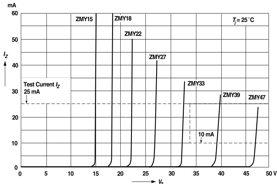
Figure 7. Breakdown Characteristics
