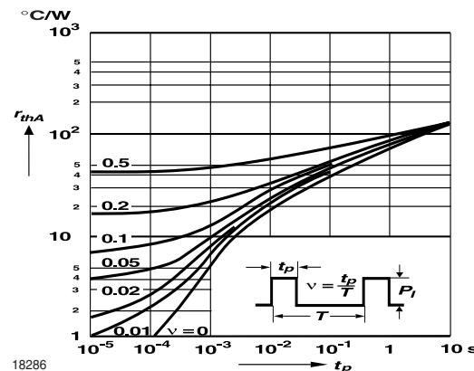
Figure 5. Pulse Thermal Resistance vs. Pulse Duration
