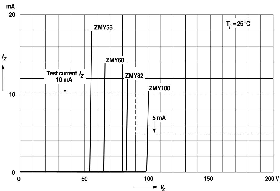
Figure 8. Breakdown Characteristics
