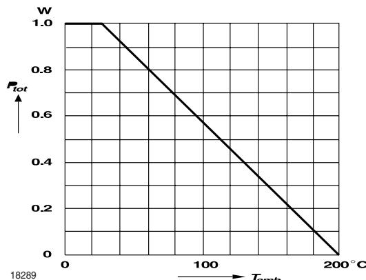
Figure 4. Admissible Power Dissipation vs. Ambient Temperature
