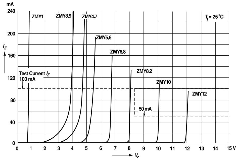
Figure 6. Breakdown Characteristics
